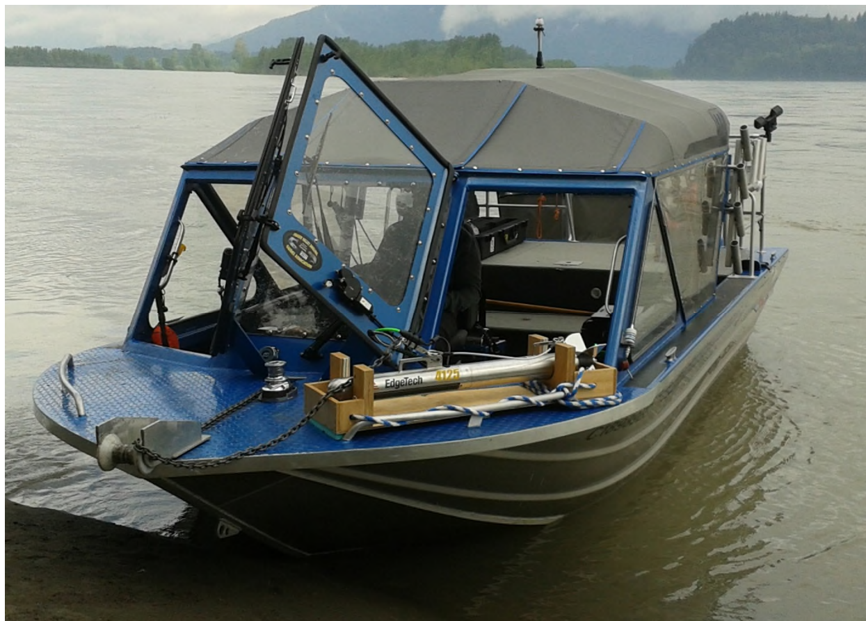
Figure 1. EdgeTech 4125 side-scan sonar setup on the bow of the survey boat.
