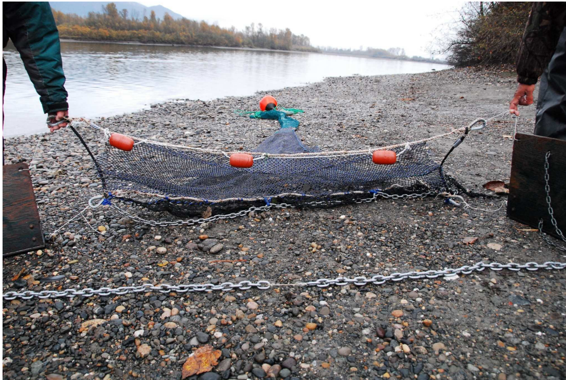
Plate 1: Front view of trawl with otter boards and 'tickler' chain, and buoy tied to the cod end. The 'breaking points', to break when badly snagged, were of 2 mm diameter nylon cord, with one of them located in the middle of the 'tickler chain' and the others as the lines between each of the otter boards and the trawl.
