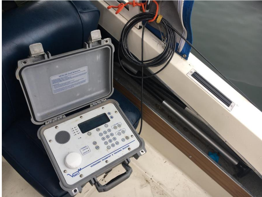
Figure 10. Placement of the Vemco VR100 hydroacoustic tag reader in the boat behind the driver (starboard side) while tracking White Sturgeon in the Fraser River.
